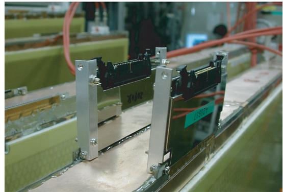
Fig. 4.14: Picture of ASD (with shield)
