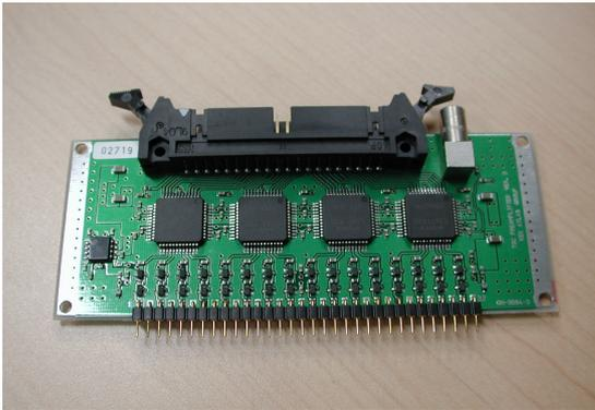
Fig. 4.13: Picture of ASD card (without shield)
