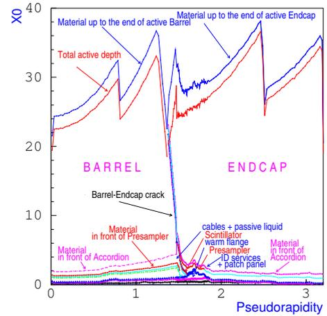
Figure 3.12: Total thickness in radiation lengths of the ATLAS EM calorimeter as a function of  $\eta$  [37].
