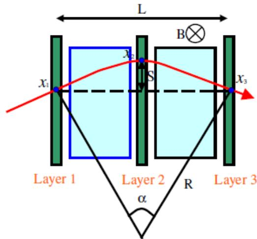
Figure 3.19: Measurement of sagitta.
