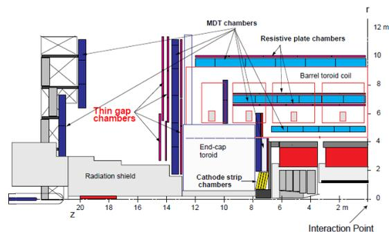
Figure 3.14: 3D muon spectrometer layout [33].
