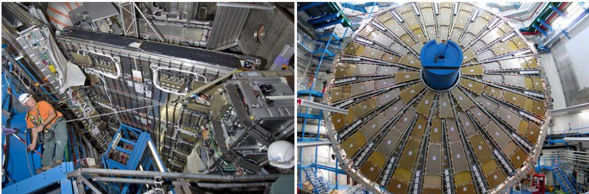
Figure 3.27: The ATLAS Muon Trigger chambers. RPC (left), TGC big wheel (right) [33].
