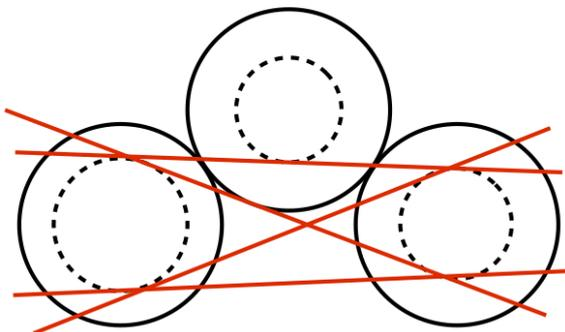
Figure 5.4: Drift circle seeds with four tangent lines
