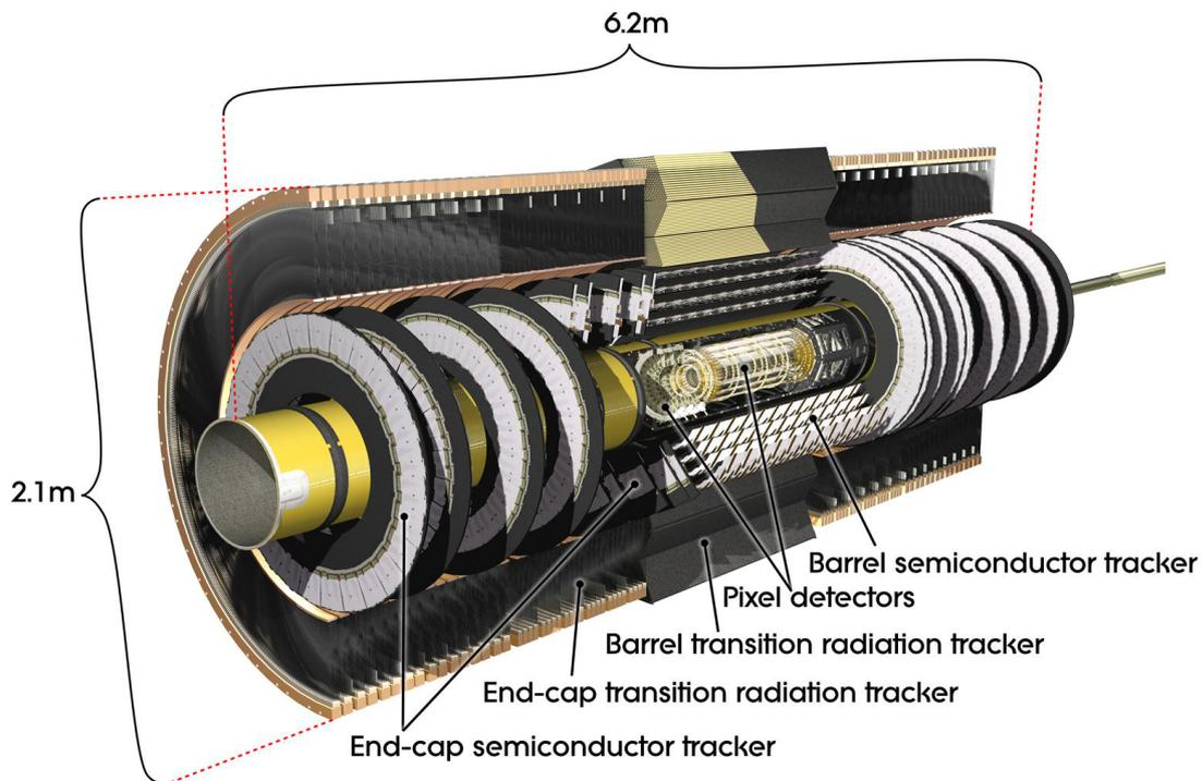
Figure 3.6: 3D overall inner detector layout [33].
