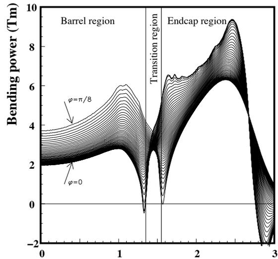
Figure 3.18: Toroid bending power  $\int Bdl$  of the azimuthal field component, integrated between the inner and outer muon station as a function of  $\eta$ [38].
