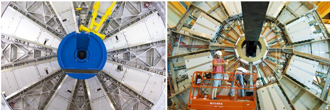
Figure 3.20: The ATLAS muon precision chambers. MDT big wheel (left), CSC small wheel (right) [33].
