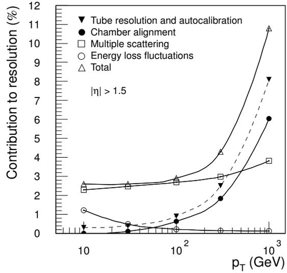
Figure 3.25:  $\Delta p_T/p_T$  as a function of  $p_T$  for muons reconstructed in the end-cap region  $\eta > 1.5$  [36].
