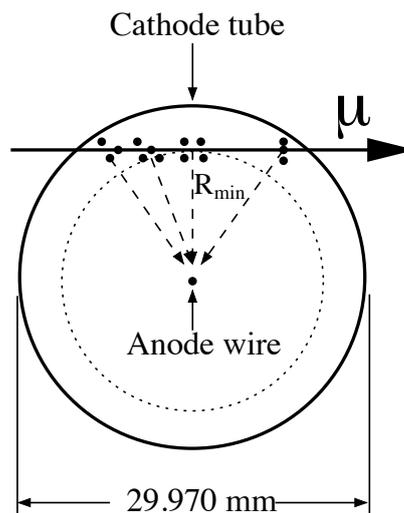
Figure 3.22: Drift tube operation in a magnetic field with curved drift pass [36].
