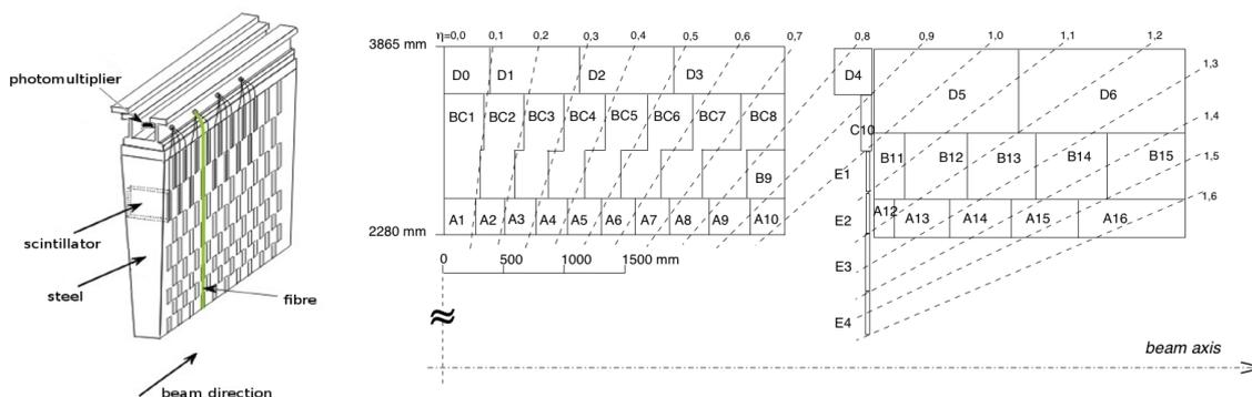
Figure 3.13: Left: a schematic display of a module, showing the passive and active material, and the optical readout system. Right: a schematic display of the cell structure in the central and extended barrel [37].
