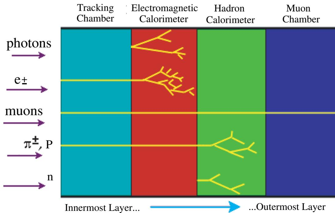
Figure 3.5: Particles' behavior in each detector
