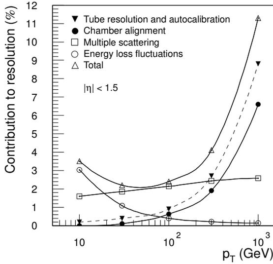
Figure 3.24:  $\Delta p_T/p_T$  as a function of  $p_T$  for muons reconstructed in the barrel region  $\eta < 1.5$  [36].
