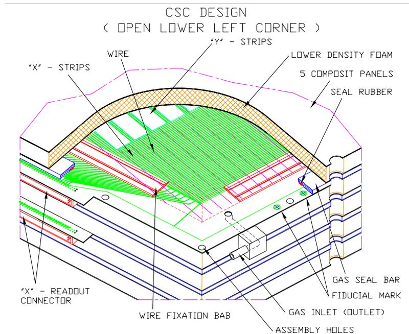
Figure 3.26: Schematic view of CSC [39].
