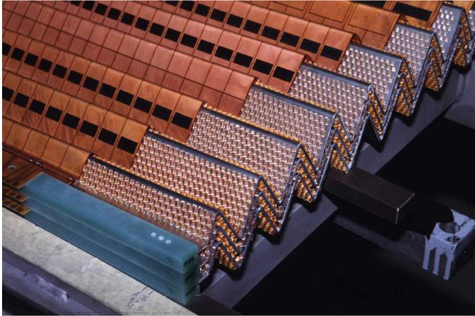
Figure 3.11: The accordion geometry of the LAr electromagnetic calorimeter [33].
