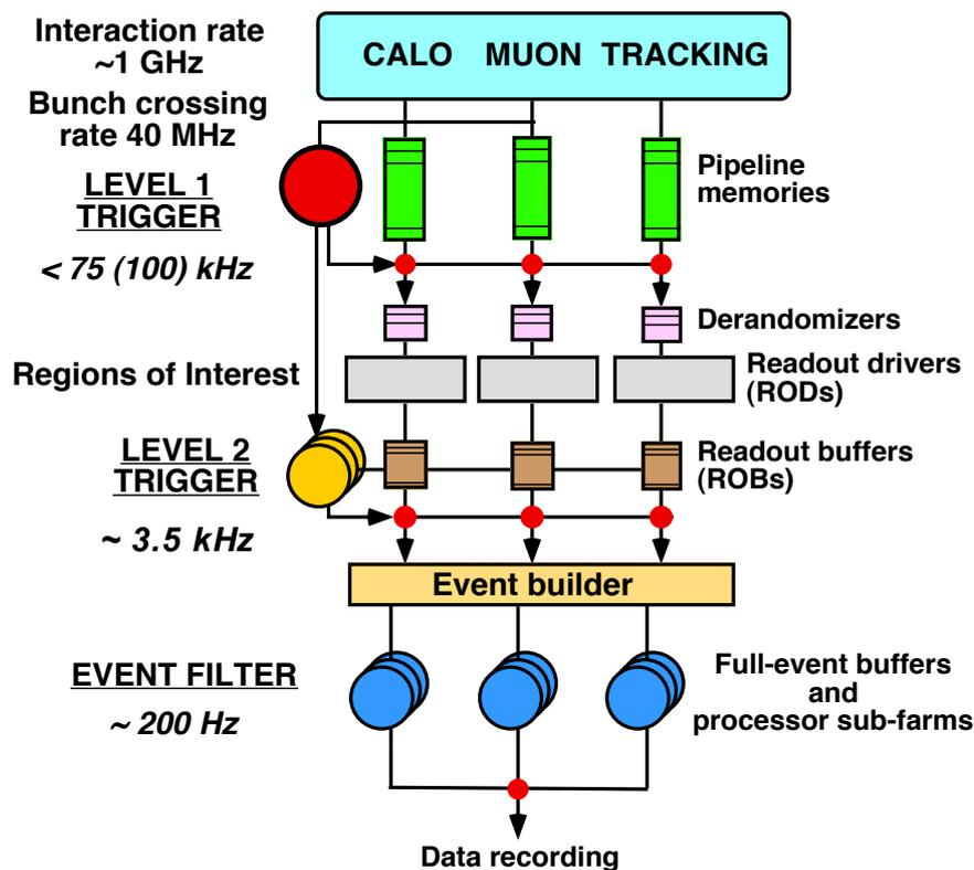
Figure 3.31: Schematic view of the ATLAS trigger system [41].
