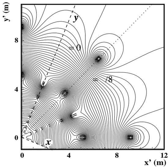
Figure 3.17: Magnetic field map in the transition region between the barrel and the endcap. The field lines in the transverse plane are shown. The coordinate system of the magnetic field is rotated by  $\frac{\pi}{8}$  with respect to the ATLAS coordinate system[38].
