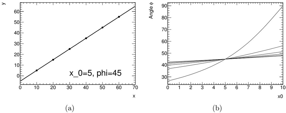
Figure 5.1: Set of points (a) and their representation in the Hough space (b).
