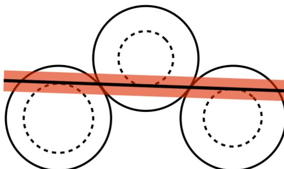
Figure 5.5: Make segment candidate by associating hits with tangent line.
