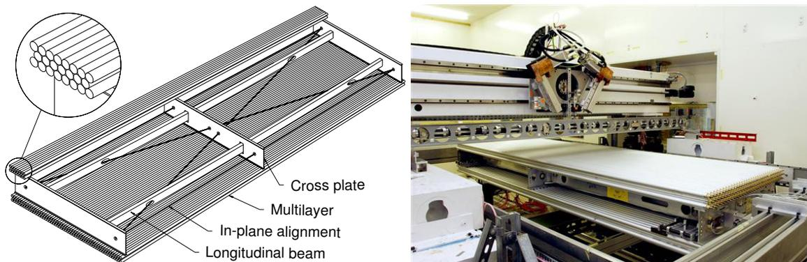
Figure 3.23: Schematic view of the MDT chamber [33][36].
