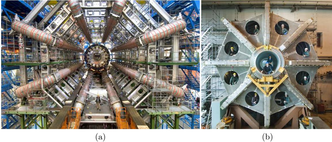
Figure 3.16: The toroidal magnets for the barrel (a) and the endcap (b) regions [33].
