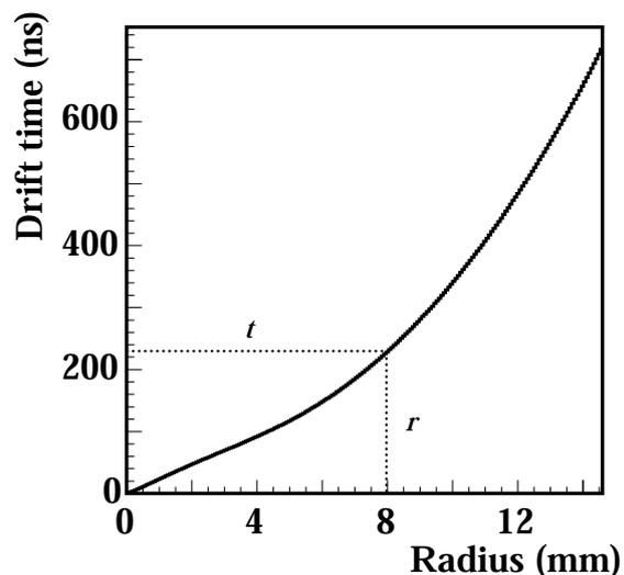
Figure 3.21: Relation between measured drift time and corresponding drift length in the absence of a magnetic field [36].
