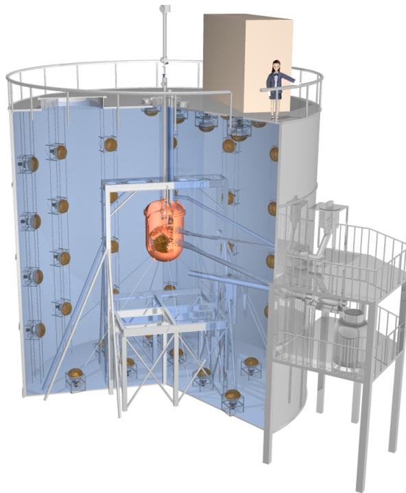
Figure 5.2: XMASS detector in the water tank
