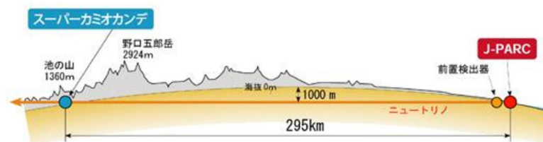
Fig. 2.1 A schematic figure of the T2K neutrino baseline, from the beamline at J-PARC through the near detectors and then 295 km underneath the main island of Japan to Super-Kamiokande.
