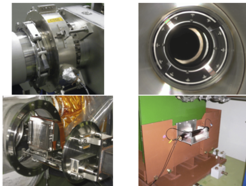
Fig. 2.6 Photographs of the primary beam line monitors. Upper left: CT. Upper right: ESM. Lower left: SSEM Lower right:BLM.
