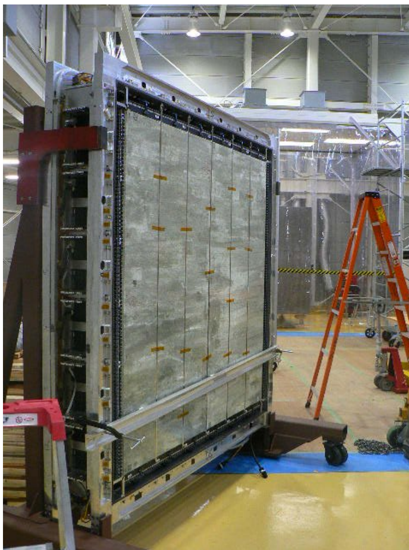
Fig. 2.20 Photograph of an FGD with the front cover removed, supported by a portable brown cart. The surface of the outermost XY scintillator module is clearly visible, along with the fiber steel steps that support its weight.
