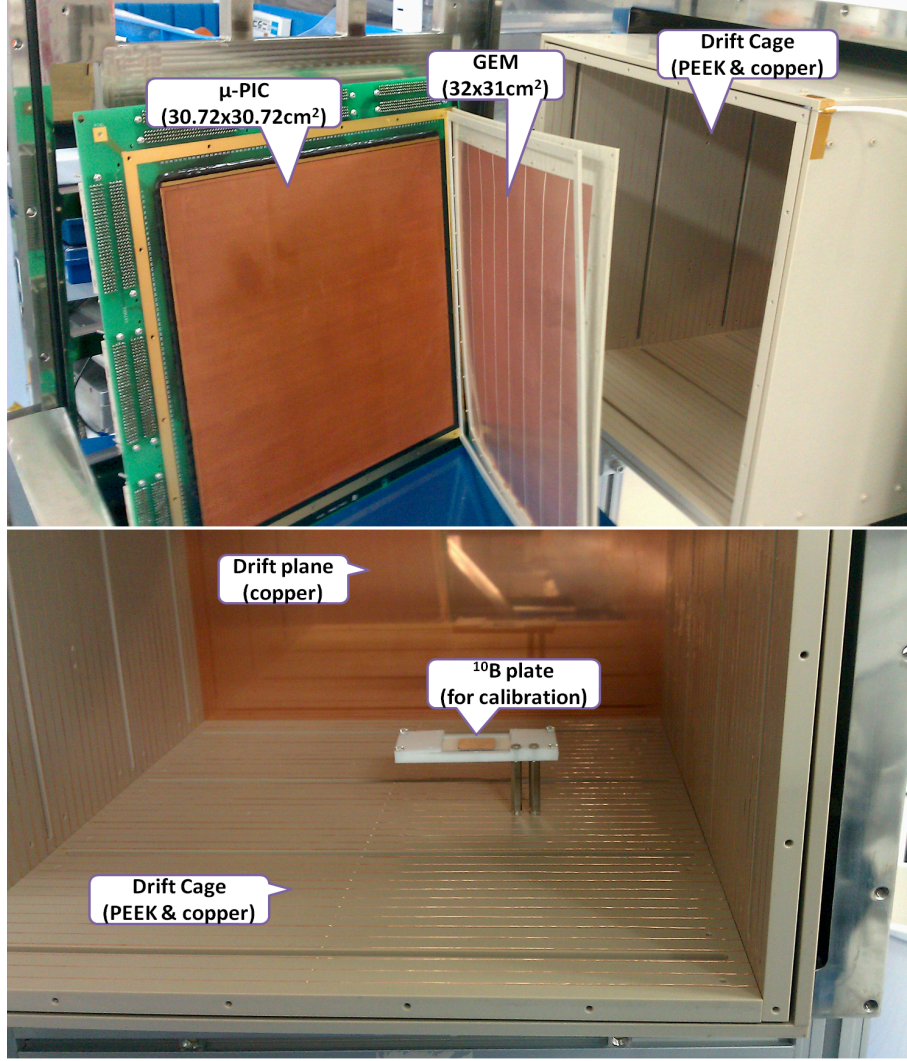
Figure 4.3: The \mu -PIC and the GEM during their installation (upper) and inner structure of \mu -TPC including the ^{10}\text{B} -evaporated glass plate (lower).
