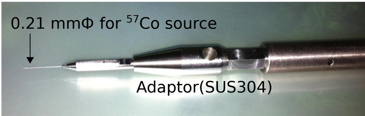
Figure 4.2: A picture of a sample of a calibration rod.  $^{57}\text{Co}$  and  $^{241}\text{Am}$  calibration sources have this shape.
