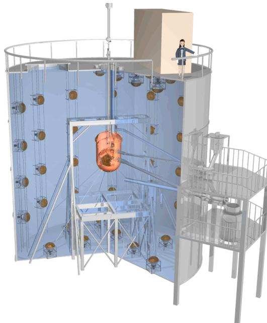
Figure 3.2: Water tank for XMASS detector. Its height and diameter are 10 m and 11 m. 20 inch PMTs are installed in the tank and work as outer detector(OD).
