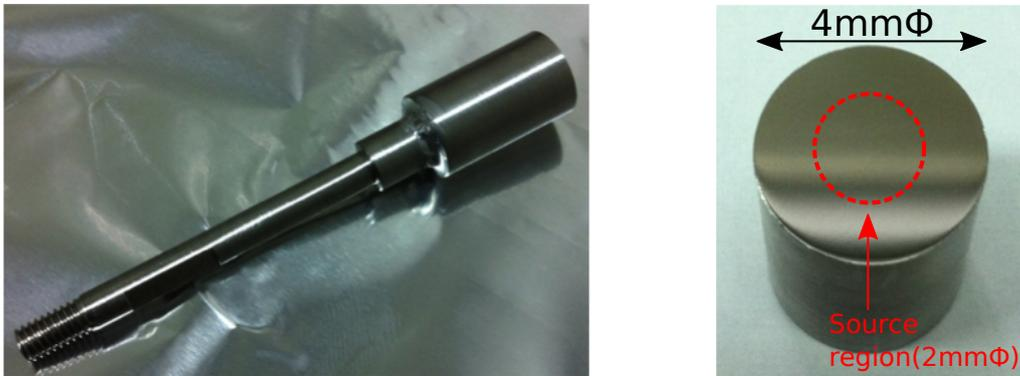
Figure 4.5: Pictures of a sample of the new  $^{55}\text{Fe}$  and  $^{241}\text{Am}$  calibration sources. Surface of the sources has a flat structure and its roughness is controlled to be less than  $1\mu\text{m}$  by buffing.
