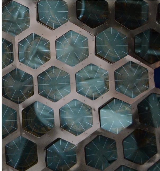
Figure 3.15: A picture of XMASS-I detector surface taken during the construction. Cu plates are attached on the detector surface.
