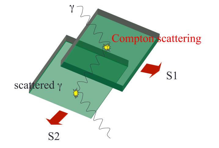
Segmented detector  $\rightarrow$  Remove Compton scattering
