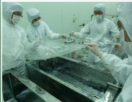
Ultra-sonic cleaning using ultra-pure water
