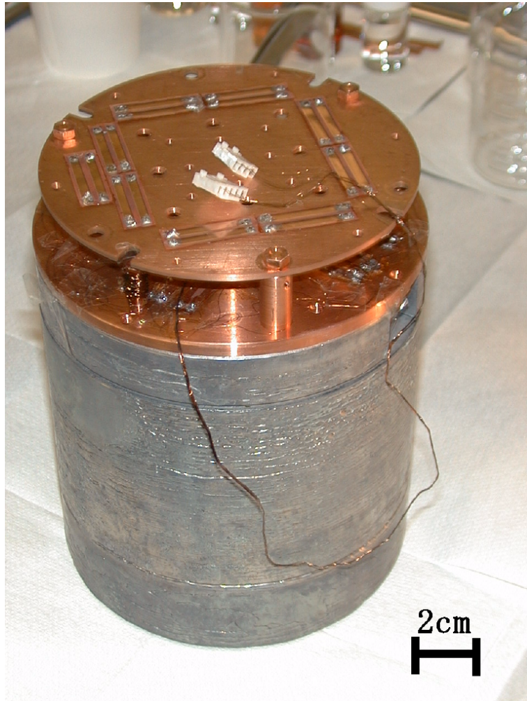
Figure 5.18: Picture of the inner shield. The bolometer array is encapsulated in the Kanazawa lead of 2cm thick.
