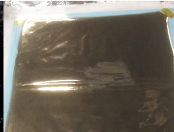
carbon sputtered EVOH sheet (for radon barrier)
