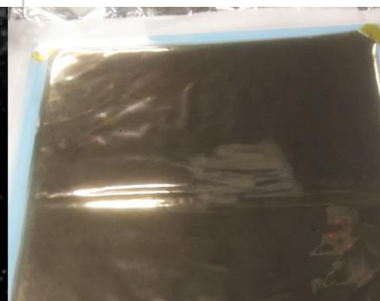
carbon sputtered EVOH sheet (for radon barrier)
