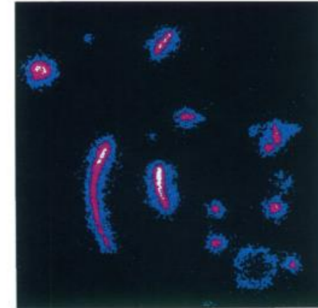
FIG. 2. A false color CCD image resulting from a ^{252}\text{Cf} neutron source. The colors black, blue, red, and white represent the order of increasing light intensity levels. The area displayed represents a 25 cm by 25 cm section of the detector plane. See the text for a description of image features.
