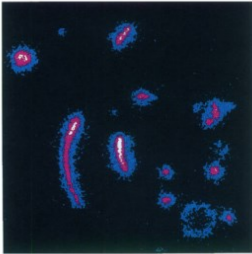
FIG. 2. A false color CCD image resulting from a ^{252}\text{Cf} neutron source. The colors black, blue, red, and white represent the order of increasing light intensity levels. The area displayed represents a 25 cm by 25 cm section of the detector plane. See the text for a description of image features.
