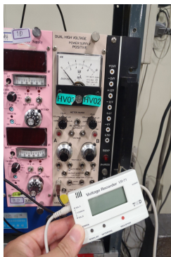
図 5.16(a) : Voltage Recorder
