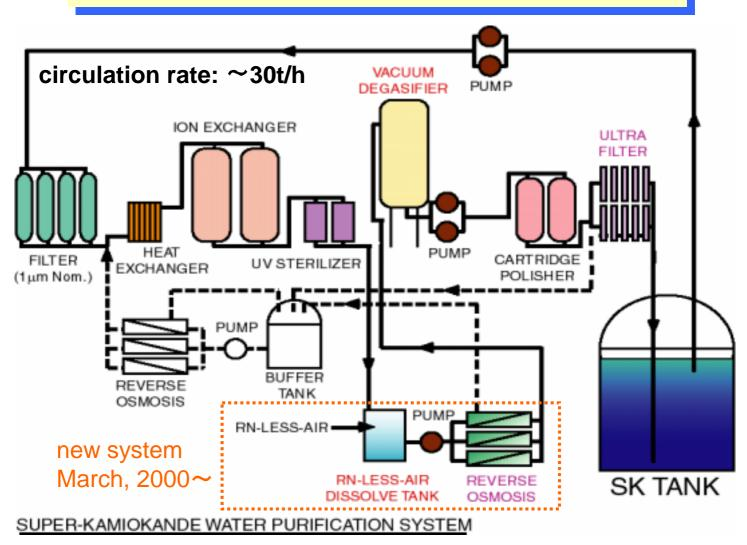
UF: ~100% remove for >100nm particles RO: remove >0.1nm particles, but not 100% → complement
