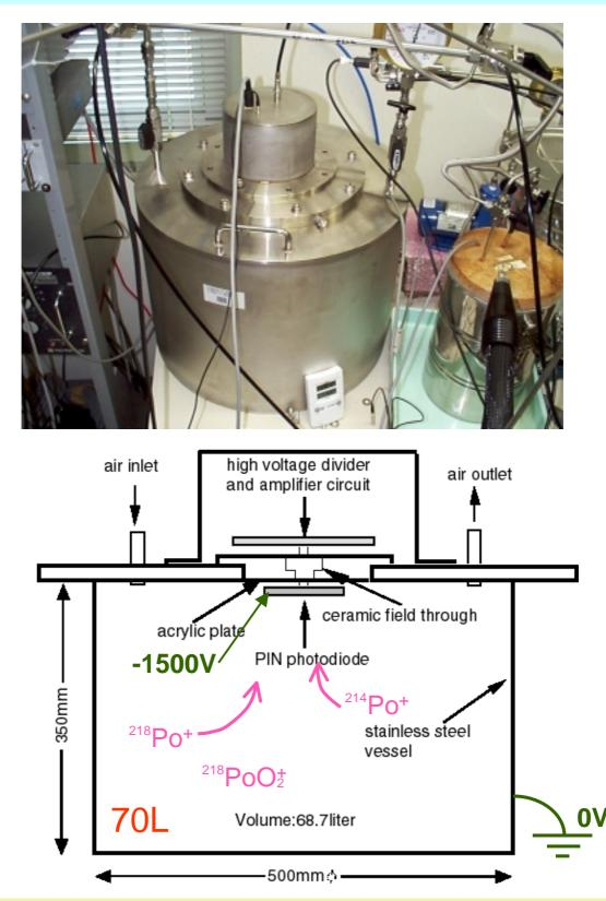
**2.2±0.4** (<sup>214</sup>Po count/day)/(mBq/m<sup>3</sup>) @0.08gH<sub>2</sub>O/m<sup>3</sup> **0.9±0.2** (<sup>214</sup>Po count/day)/(mBq/m<sup>3</sup>) @11gH<sub>2</sub>O/m<sup>3</sup>
