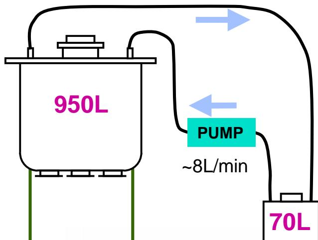
Connect 950L and 70L Rn detectors, then compare the count rates for each detector.
