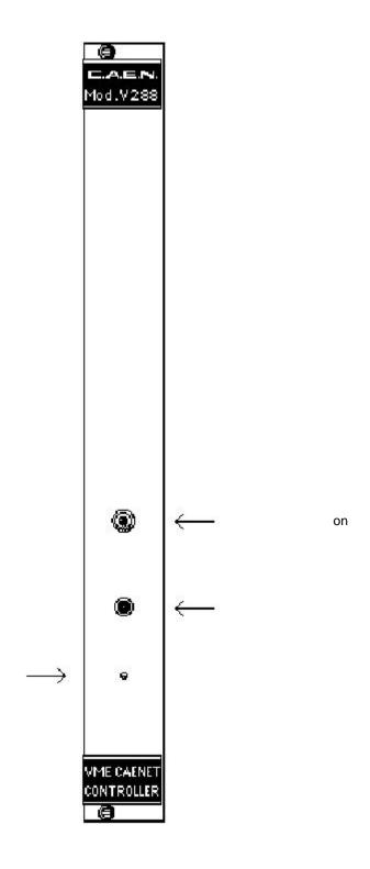
Fig 2.1 Mod. V288 Front Panel
