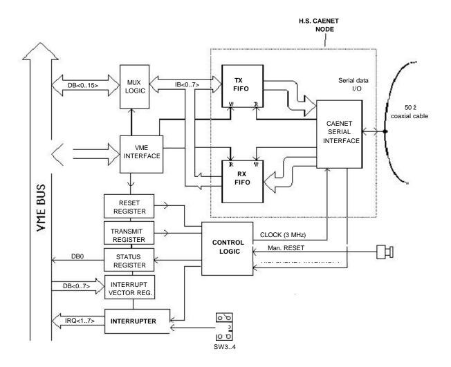
Fig 1.1 Mod. V288 block diagram
