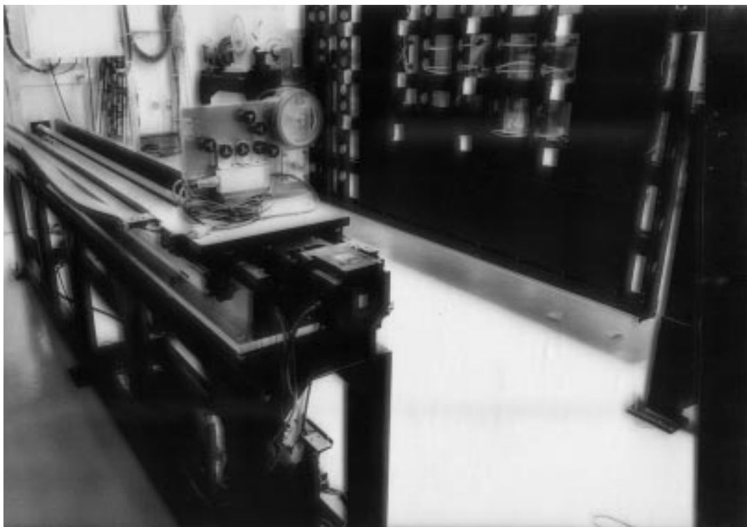
Figure 3-4 Winding machine at KEK showing the attachment vacuum system.
